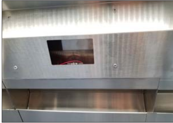
Figure 2: Extractor Positioning Switch Access Opening with Switch Housing Cover Removed
