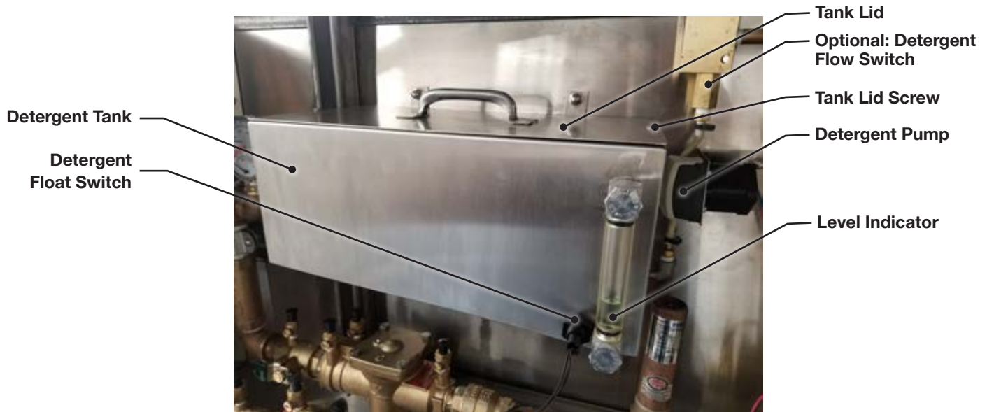
Figure 29: Detergent Injection System
