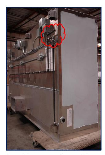
All pipe and conduit field connections will be factory piped towards the most accessible point of the hood to ease field installation. (See clouded areas)
