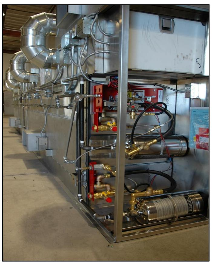
FSS cabinets will be piped and fully assembled at the factory with all applicable components such as control head(s)/automan(s), (4) microswitches, gas cartridge(s), agent tank(s), mounting bracket(s), tank strap(s), corner pulley(s), and copper tubing. Unions are also provided on tank distribution connections for ease of removal and installation of agent tank(s).
