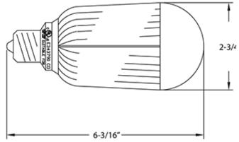
Energy-saving LED light for Commercial Kitchen Hood applications with maximized light output at a fraction of the wattage consumed by standard incandescent and fluorescent lights.
